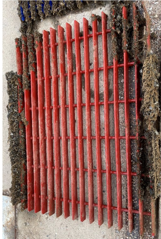
Figure 32: Sigmaglide 1290 dynamic test grate after 2 years in field testing during July 2022 inspection.
