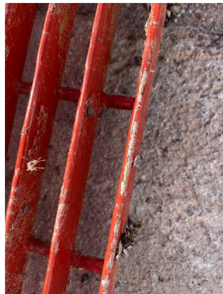
Figure 8: Abrasion style damage of Jotun Sealion Repulse test grate.
