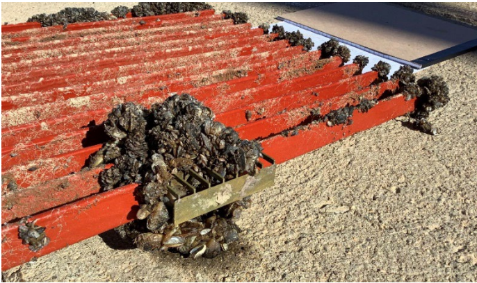
Figure 54: Z-Alloy fish screen during January 2022 inspection. All fouling appeared to be attached to zip-ties securing screen to larger test grate.
