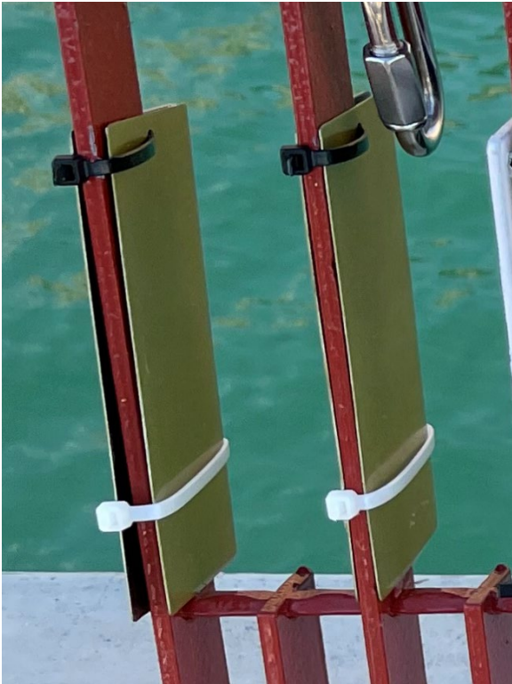
Figure 2: Popspeed panels on experimental rack for dynamic testing prior to January 2022 installation.
