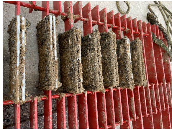
Figure 90: PNNL panels on experimental rack after approximately 6 months of testing. Minor mussel fouling and some buildup of colonial hydroid. Formulations 3 through 10 (left to right).
