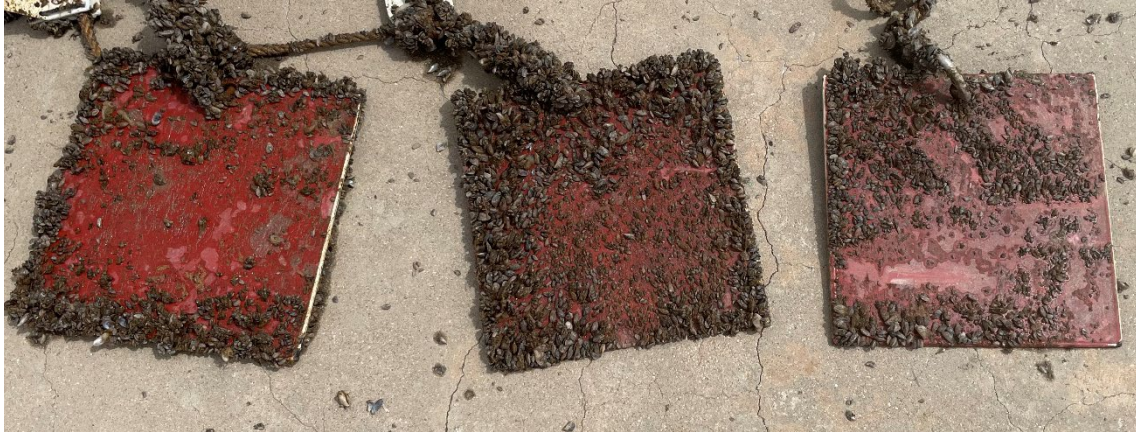
Figure 12: Jotun Sealion Resilient static test plates during July 2022 inspection with the surface partially fouled with mussels.
