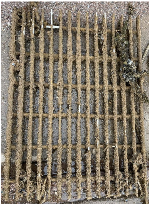
Figure 23: NuSil 9707 test grate during July 2022 inspection. Surface is 100% covered with colonial hydroid but no mussel fouling.
