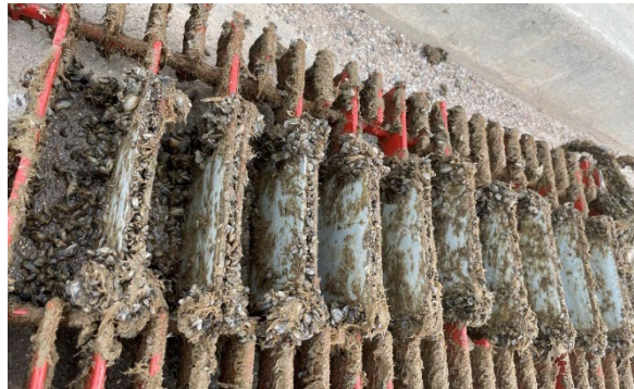
Figure 76: From left to right Formulation A, B, and C with various degrees of fouling during July 2022 inspection.
