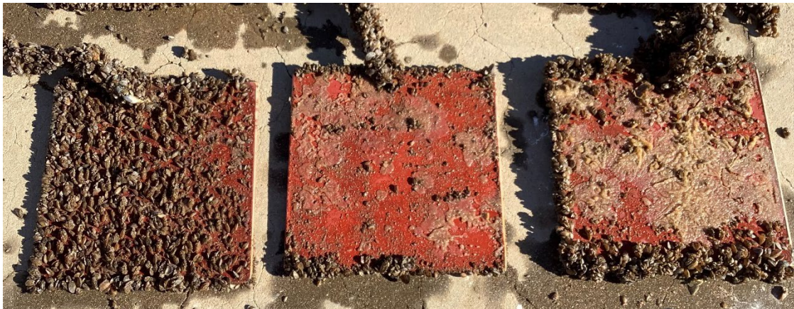
Figure 11: Jotun Sealion Resilient quasi-static test plates with mussel and sponge organism fouling during January 2022 inspection.
