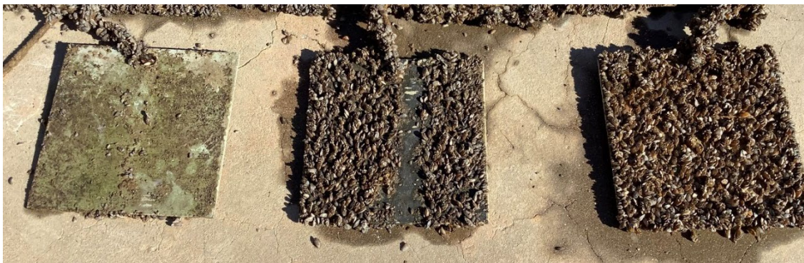
Figure 18: Silicone Solutions static test plates: F-23 (left), SS3000 (middle), and 5000A (right).
