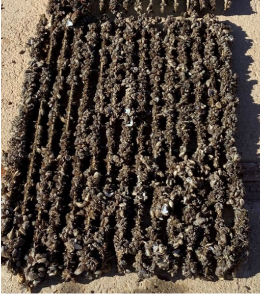
Figure 19: 5000A dynamic test grate during heavily fouled with mussels during January 2022 inspection.
