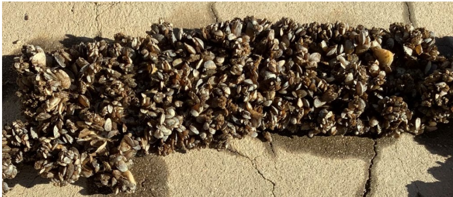
Figure 69: NDSU 3 static test panel completely fouled January 2022 inspection.
