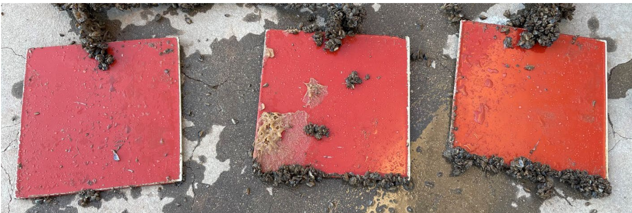
Figure 5: Quasi-static test plates for Jotun Sealion Repulse. Fouling only on edges due to damaged coating.
