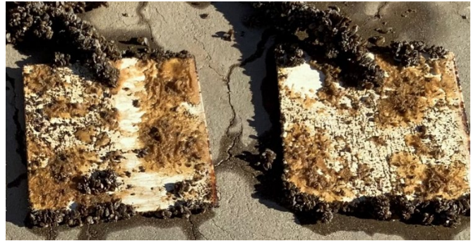
Figure 22: NuSil 9707 static plates during January 2022 inspection. Surface is fouled with sponge organism and mussel fouling is only at edges where coating is damaged.
