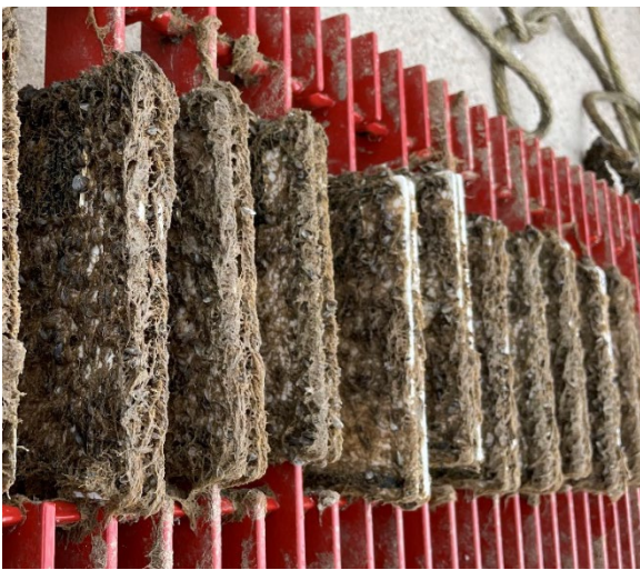
Figure 89: PNNL panels on experimental rack after approximately 6 months of testing. Minor mussel fouling and some buildup of colonial hydroid.
