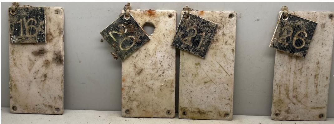
Figure 100: PNNL formulations 4 (coupon 16), 5 (coupon 20 and 21), and 6 (coupon 26) coupons that were removed from testing.
