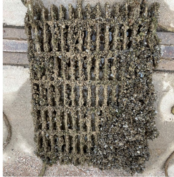
Figure 20: Silicone Solutions 5000A dynamic test grate during July 2022 inspection. Part of the grate is densely fouled with mussels and the remainder of the grate is fouled with mussels and the colonial hydroids.
