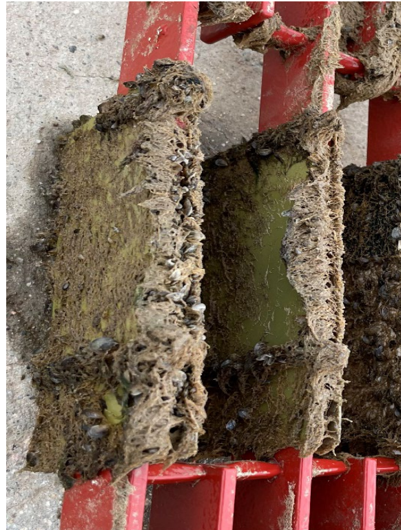
Figure 3: Popspeed after six months in dynamic testing condition. Some accumulation of the colonial hydroid on surface. Mussels are attached to zip ties and not adhered to coated surface.
