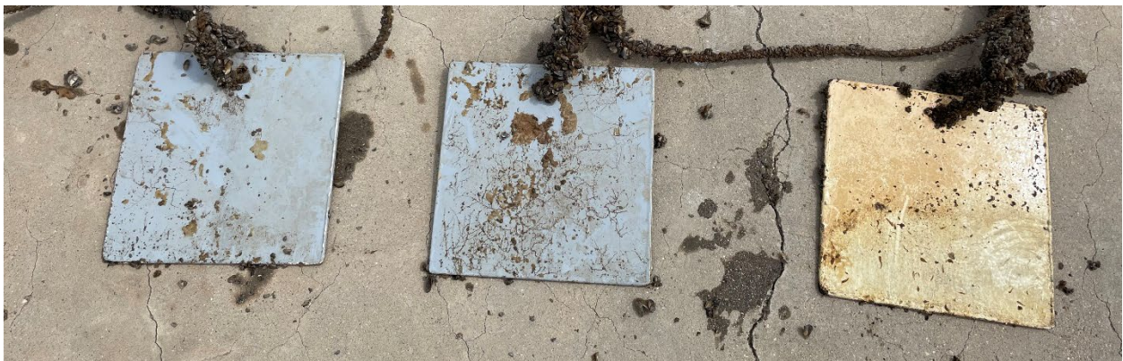
Figure 43: Intersleek 1425 quasi-static test plates. No mussel fouling and small amounts of sponge and hydroid present during July 2022 inspection.
