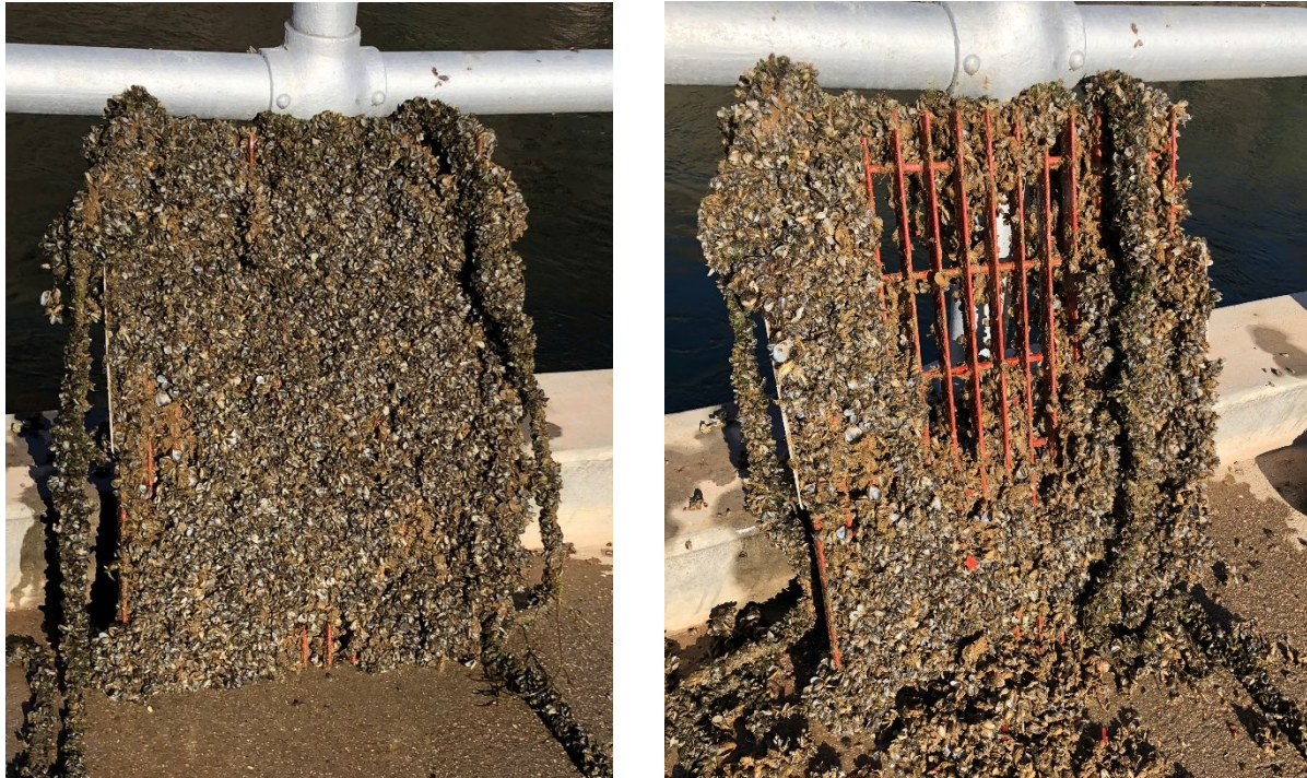
Figure 9: Jotun Sealion Resilient During 2019 inspection. 100% fouled before cleaning (left) and partially cleaned (right).
