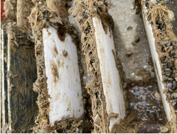
Figure 77: Formulation E after cleaning during July 2022 inspection.
