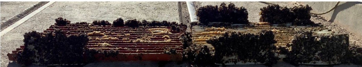
Figure 64: NDSU 7 (left), NDSU 5 (middle), and NDSU 4 (right) in dynamic testing conditions. NDSU 6 was lost during testing and one panel of NDSU 7 was lost also.
