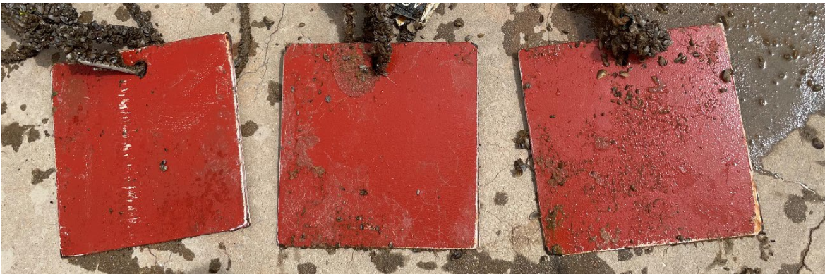
Figure 52: Hempel X3 static test plates during July 2022 inspection. One plate appears to have abrasion damage in the center of the plate caused by the rope it suspends from.
