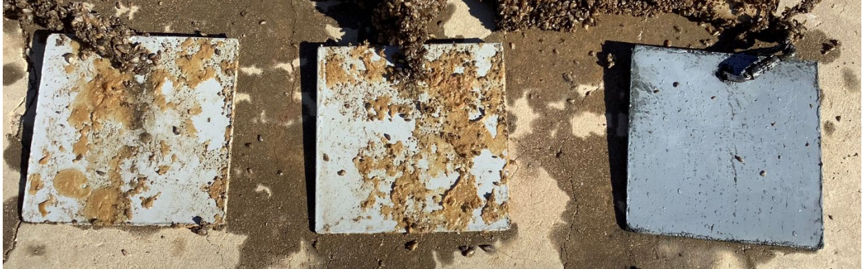
Figure 42: Intersleek 1425 quasi-static test panels with two panels being slightly fouled with sponge organism during January 2022 inspection.
