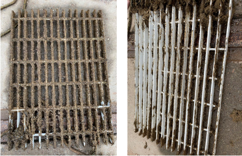
Figure 29: Before and after cleaning photos of Sigmaglide 890 dynamic test grate during July 2022 inspection. No mussel fouling but surface covered in colonial hydroid.
