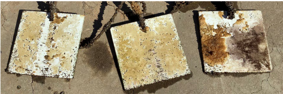
Figure 27: Static test plates Sigmaglidle 890. Fouled with sponge organism over most of the surface and one plate is stained with a dark color from an unknown source.
