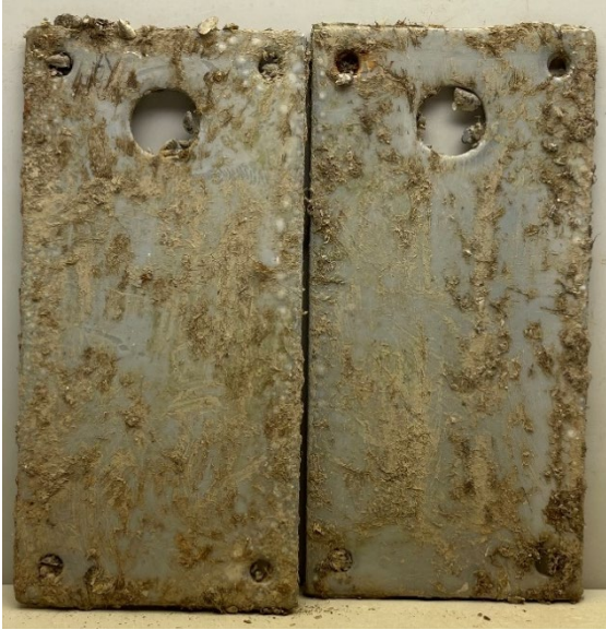
Figure 81: Adaptive Surface Technologies' Formulation A after removal from testing.
