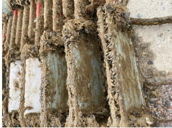
Figure 78: Formulation E and G after cleaning during July 2022 inspection.
