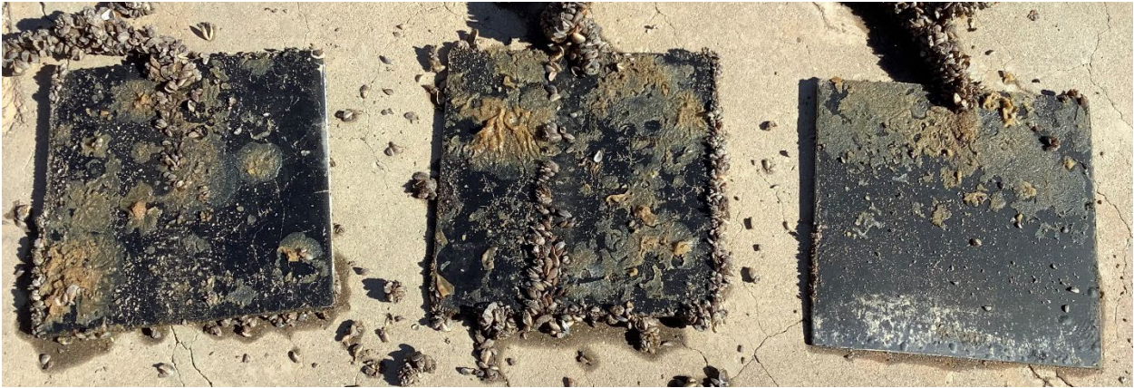
Figure 45: BioClean quasi-static test panels that are slightly fouled with both mussels and sponge organism during January 2022 inspection.
