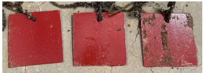
Figure 34: Sigmaglide 1290 static plates after 2 years of testing. There is no mussel fouling.
