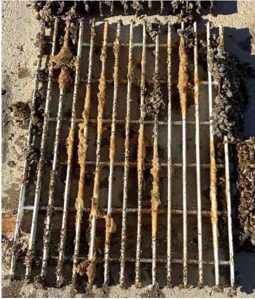
Figure 26: Sigmaglidle 890 during January 2022 inspection. Surface is lightly fouled with mostly a sponge organism and minimal mussel fouling.
