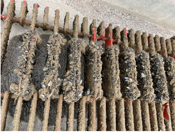
Figure 73: From left to right Formulation A, B, and C with various degrees of fouling during July 2022 inspection.
