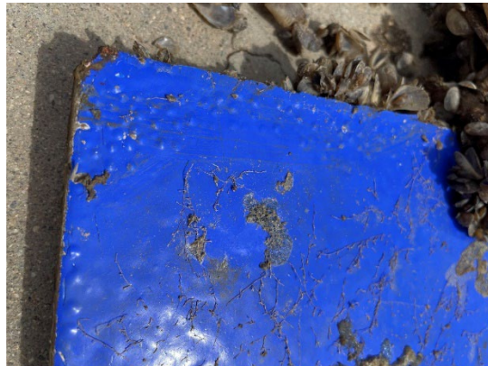
Figure 41: InterSleek 970 static plates during the July 2022 inspection with blistering observed around the edges.
