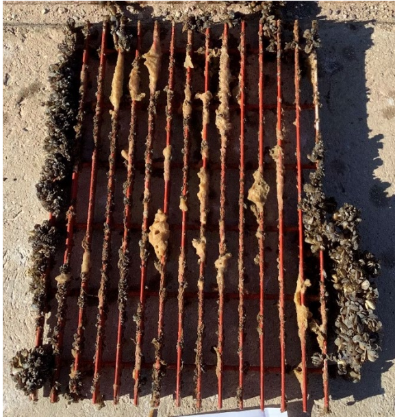
Figure 49: Hempel X3 test grate that is fouled with some mussels and sponge organism during January 2022 inspection.
