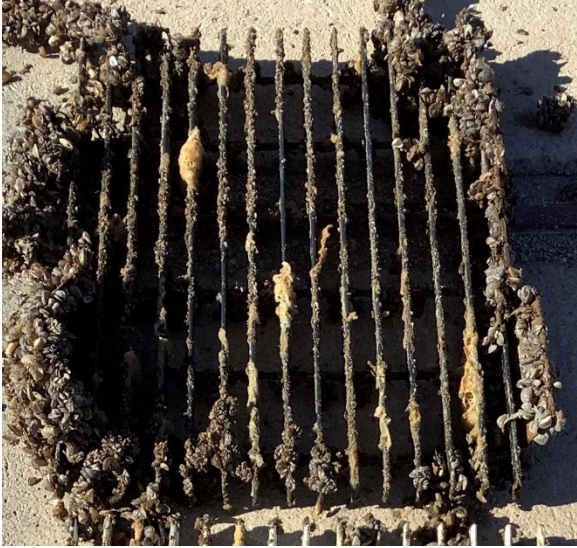
Figure 44: BioClean flowing water test grate during January 2022 inspection. Light fouling of sponge organism and mussels.
