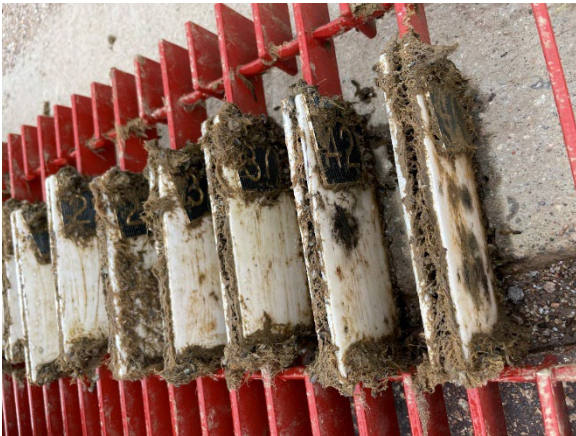
Figure 91: Panels after cleaning. Some of the black spots can be seen on the two right panels, 40 and 42.
