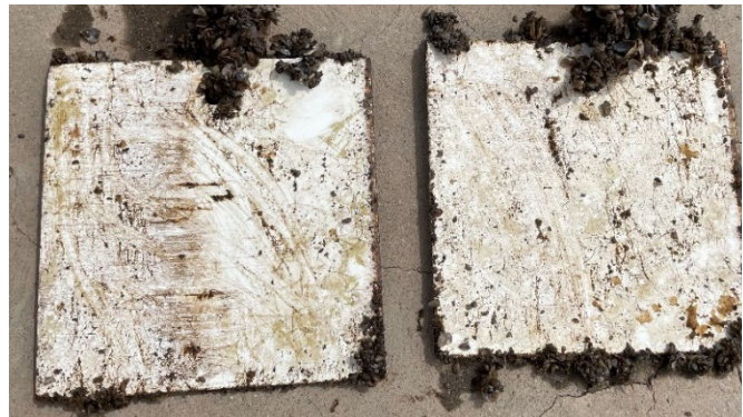
Figure 24: NuSil 9707 static plates during July 2022 inspection. Surface is free of fouling except for edges where coating is damaged.
