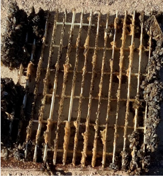
Figure 21: NuSil 9707 test grate during January 2022 inspection. Grate is fouled with sponge organism but no mussels.
