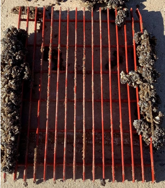
Figure 31: Sigmaglide 1290 after 1.5 years in flowing water during January 2022 inspection.
