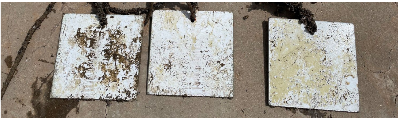
Figure 28: Static test plates Sigmaglidle 890. Little fouling from sponge organism and no mussel attachment.
