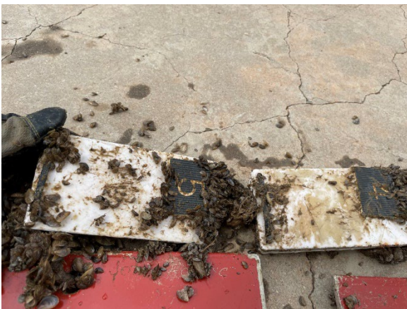
Figure 95: Formulation 1 panels in static testing. Less than 5% fouled with mussels and some sponge organism build up.
