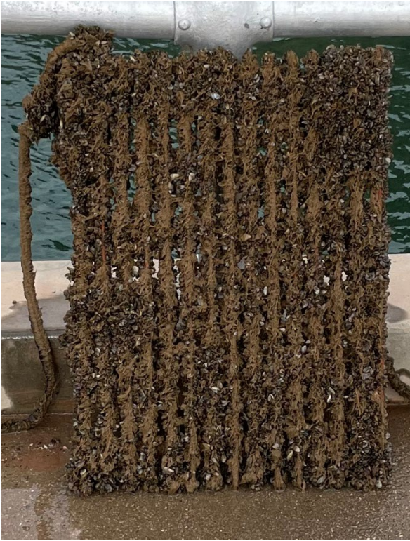
Figure 10: Jotun Sealion Resilient during July 2022 inspection with large amounts of colonial hydroid and mussel fouling.
