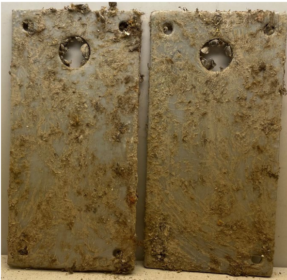
Figure 83: Adaptive Surface Technologies' Formulation C after removal from testing.
