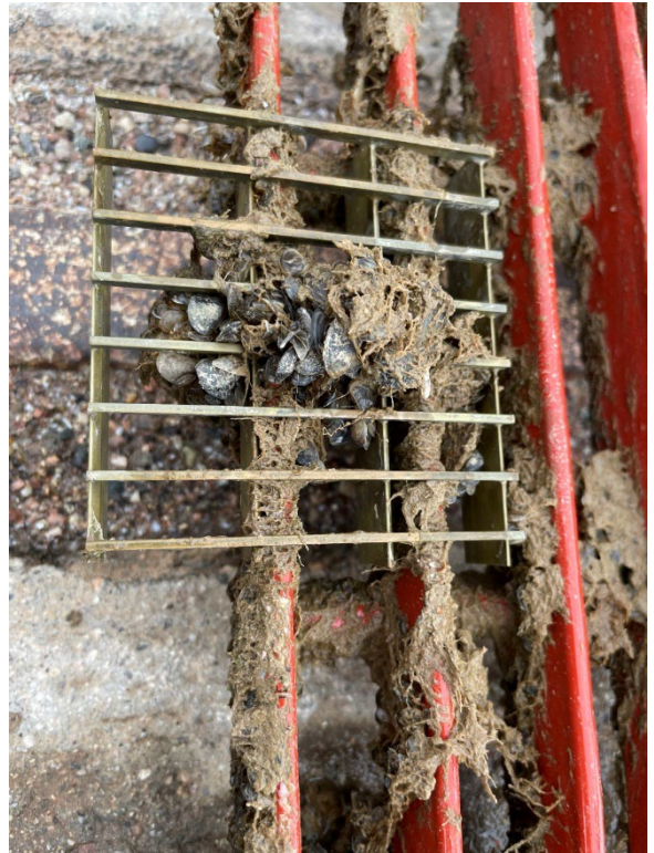
Figure 55: Z-Alloy fish screen at July 2022 inspection. All fouling is on zip-tie securing the sample.
