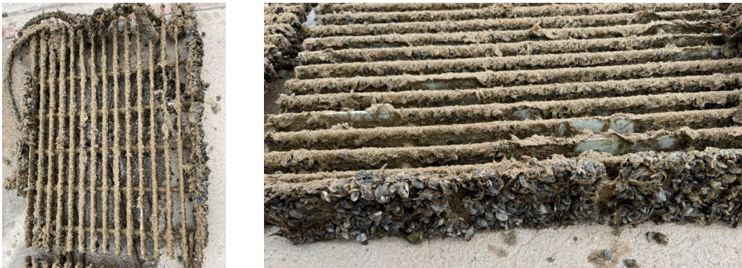
Figure 17: Top and side view of Silicone Solutions F-23 during July 2022 inspection. Minimal fouling of mussels but covered with
