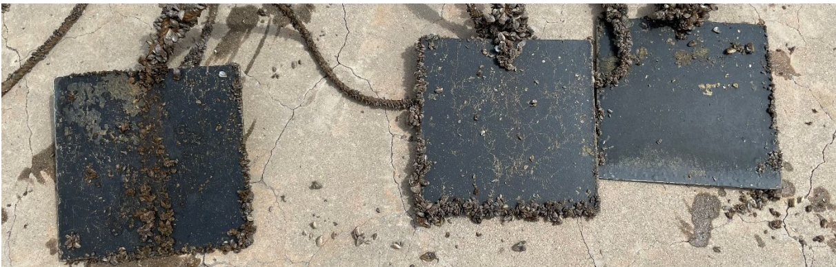
Figure 46: BioClean static test plates during July 2022 inspection.
