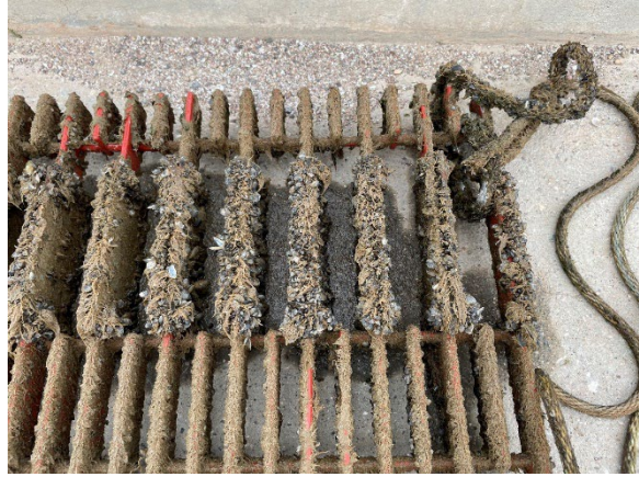
Figure 74: From left to right formulations B, C, and D with different degrees of fouling during July 2022 inspection.
