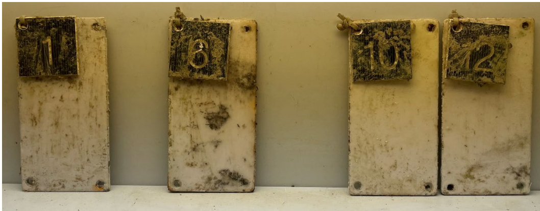
Figure 99: PNNL Formulations 1 (coupon 1), 2 (coupon 6), and 3 (coupon 10 and 12) coupons that were removed from testing.
